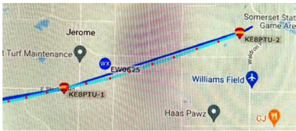
Example 2. APRS.fi website demonstrating that “frequent” RF beacons (red dots), from the -2 SSID balloon, can be uploaded onto APRS.fi without incurring network congestion.
